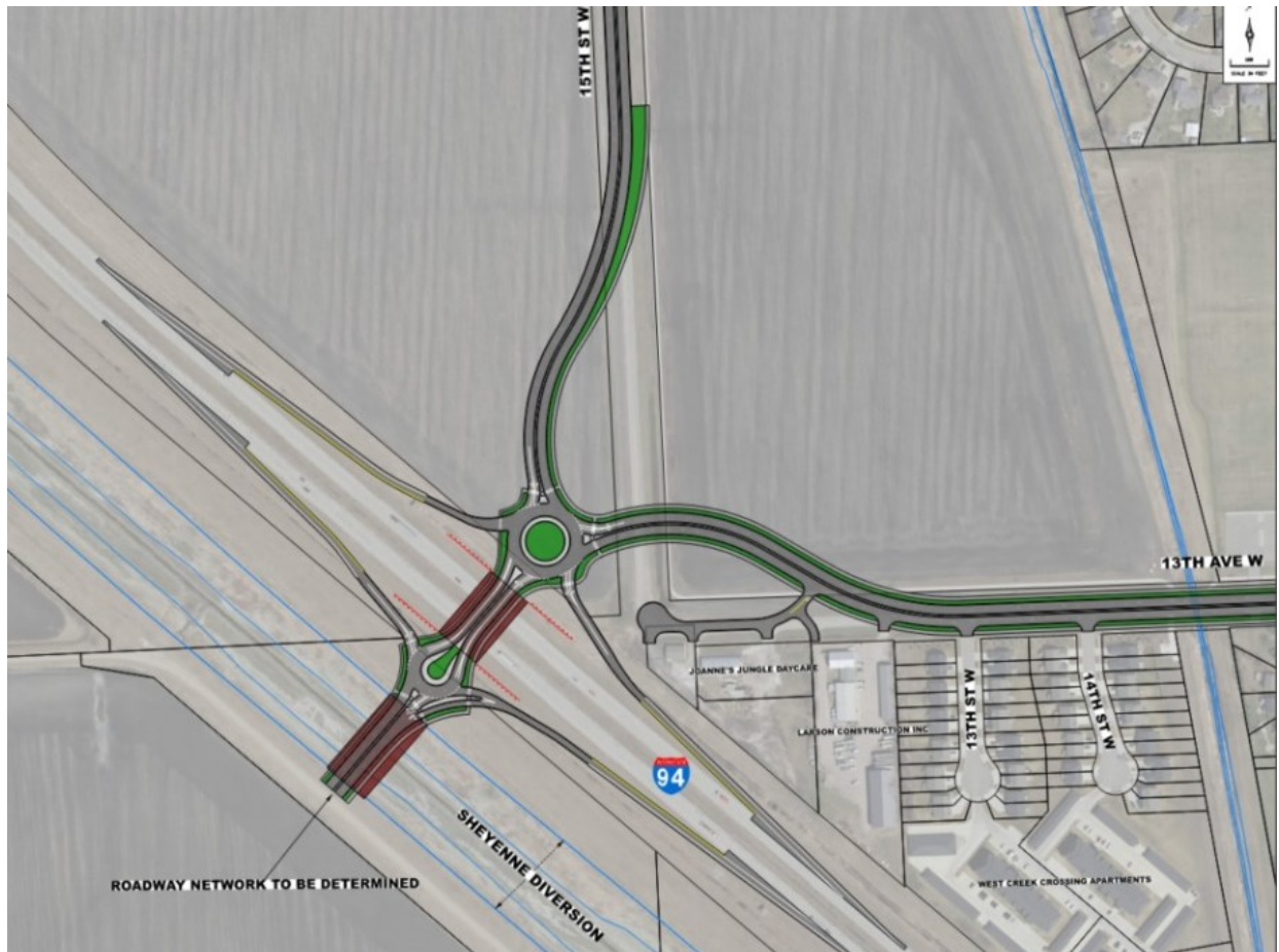
Figure 4.9 – 15 th Street and 13 th Avenue Roundabout Interchange
