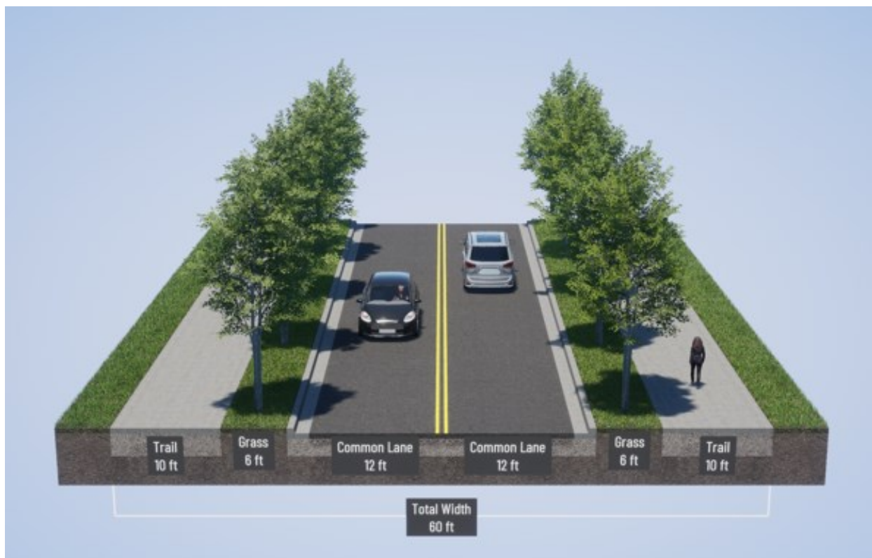
Figure 3.6 - Mixed Use Arterial Typical Section
