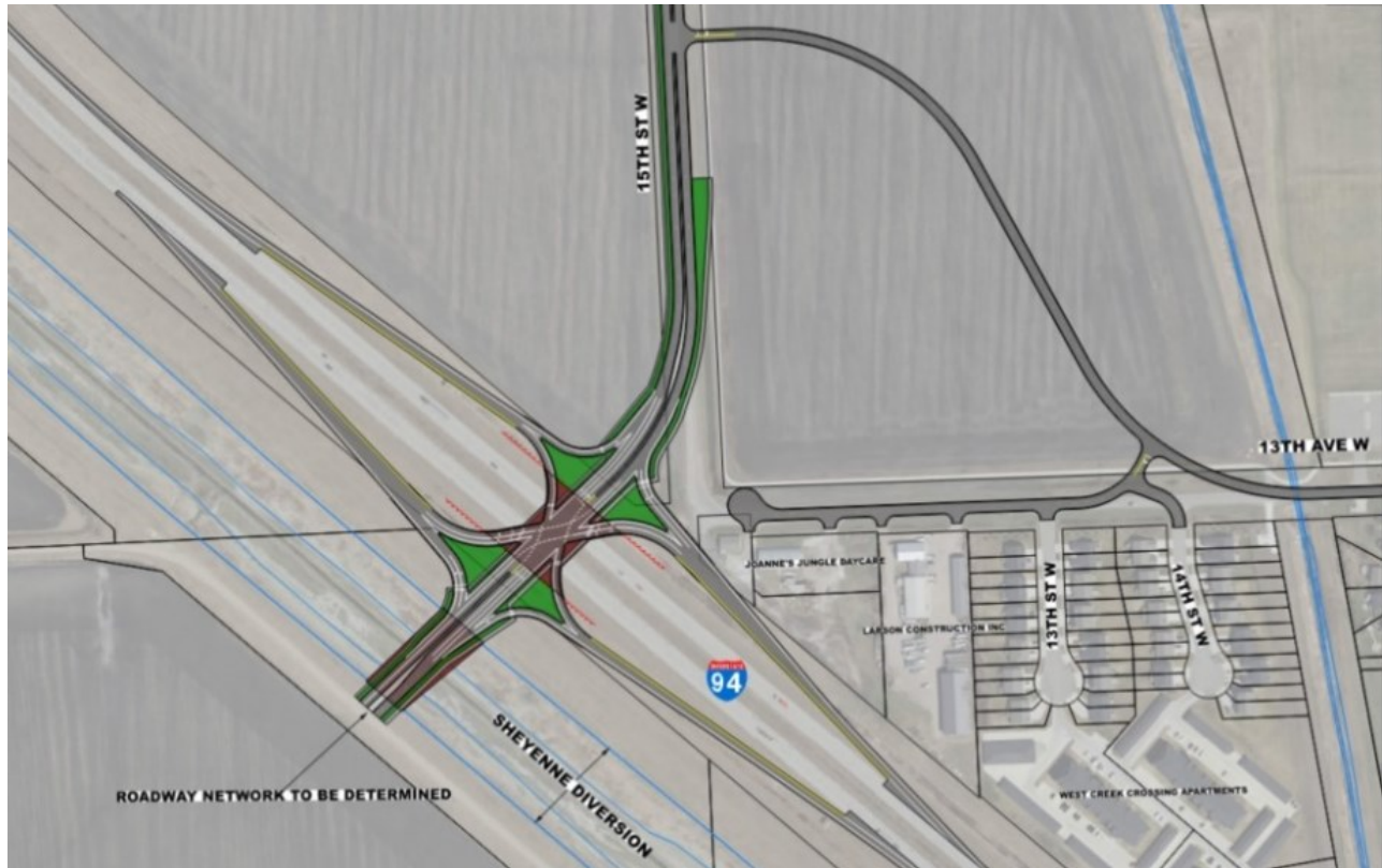
Figure 4.5 – 13 th Ave/15 th St Single Point Urban Interchange
