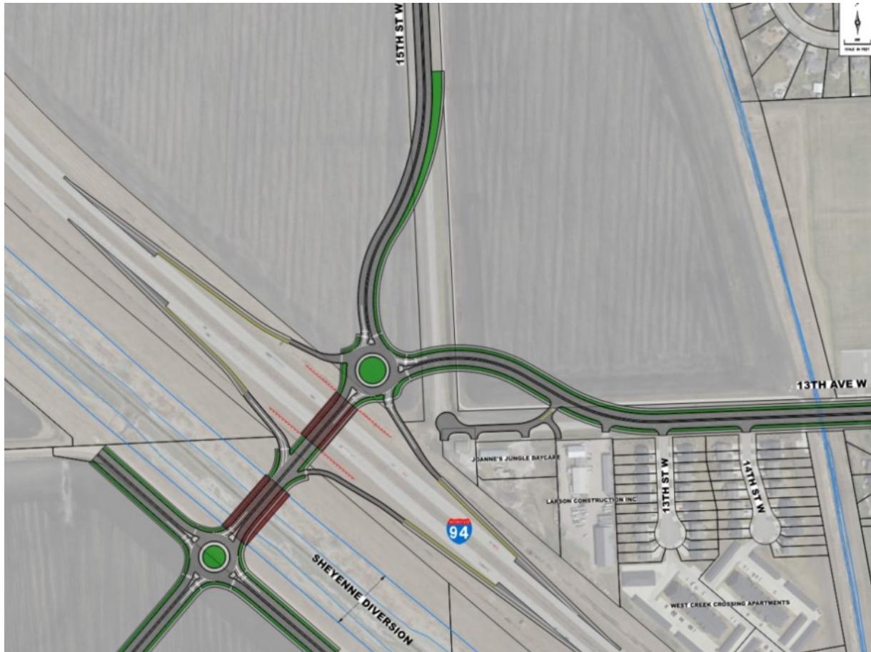
Figure 4.10 – 15 th Street and 13 th Avenue Diverted Roundabout Interchange
