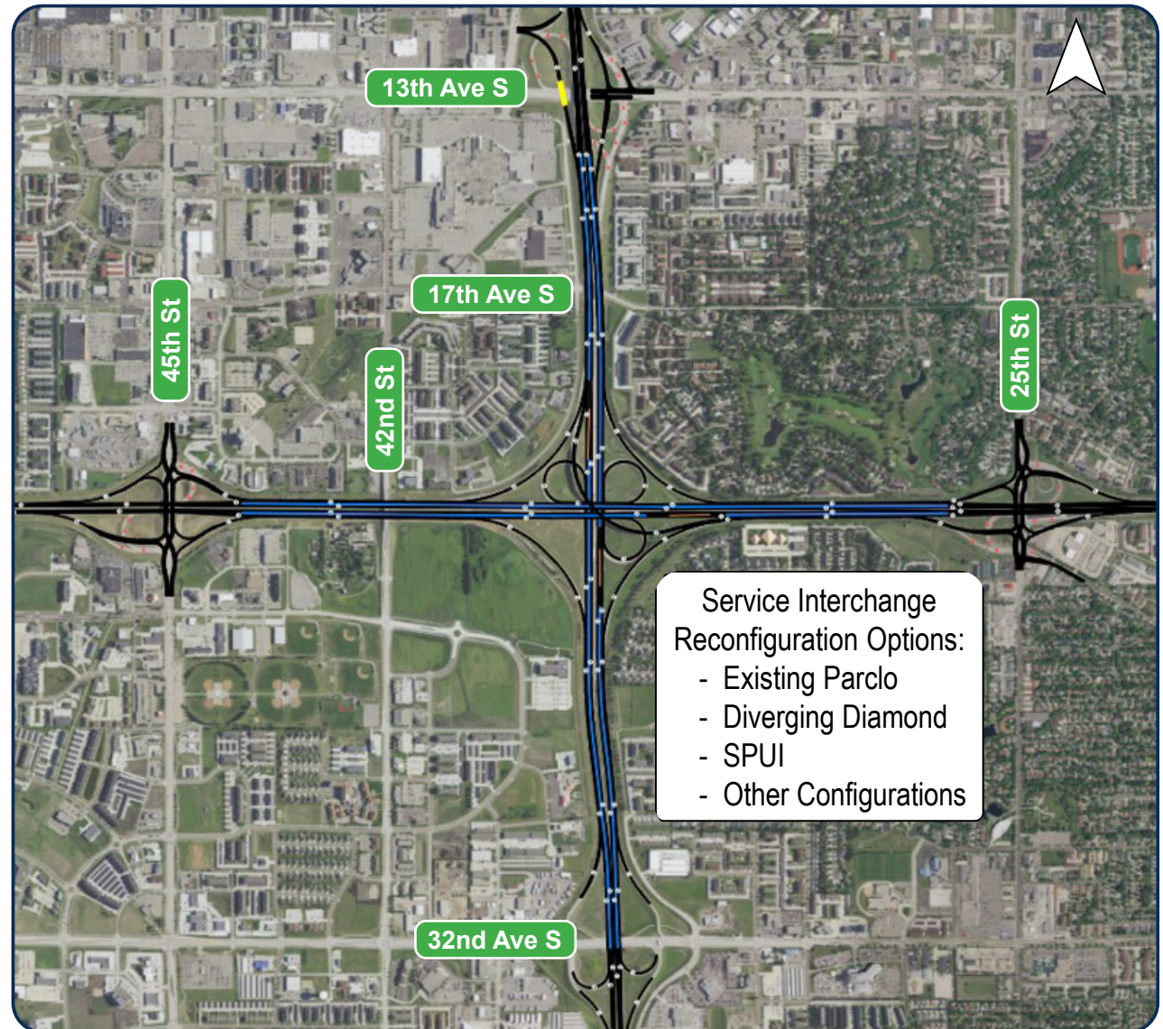
Figure 4.1. Collector-Distributor Road Strategy
