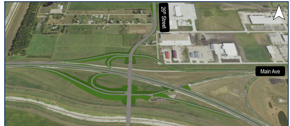
Figure 4.4. Main Avenue & 26th Street Interchange Concept
