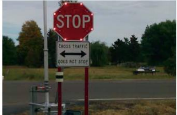
Figure 3-9. LED Stop Sign
