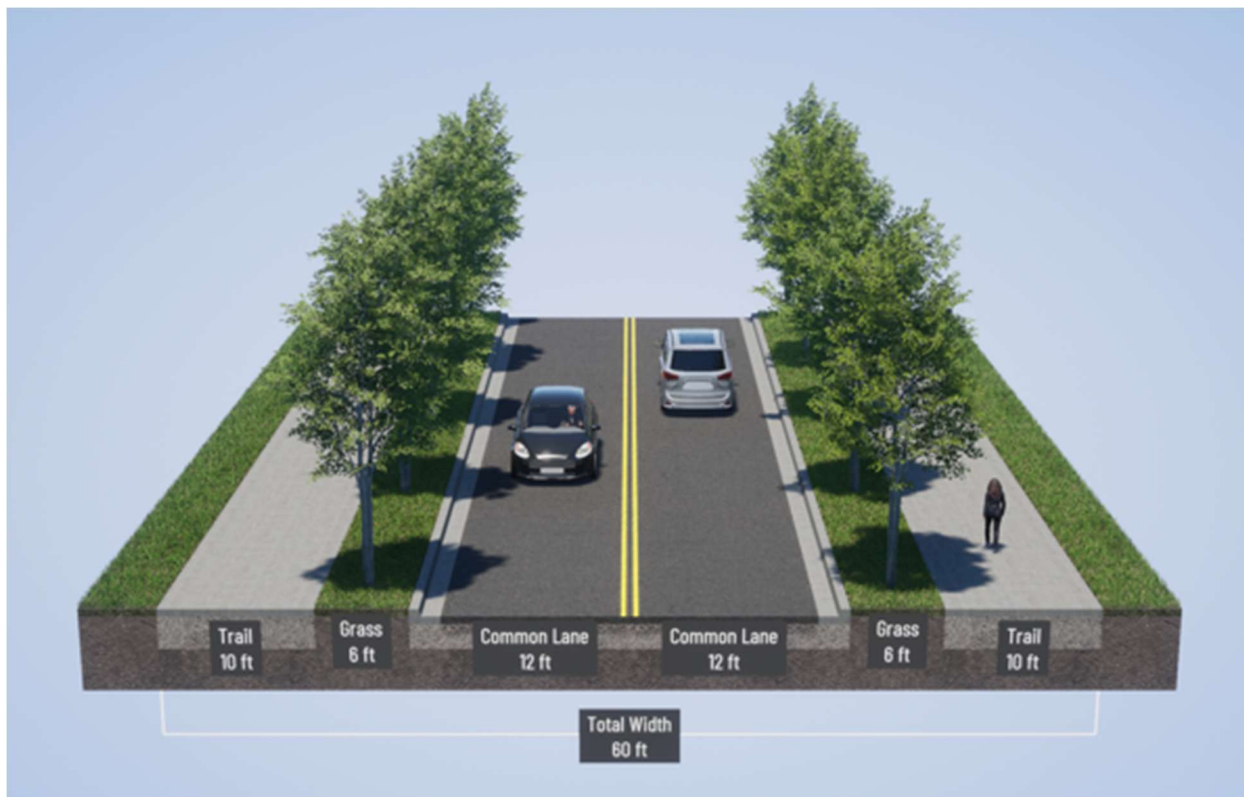
Figure 3.6 - Mixed Use Arterial Typical Section
