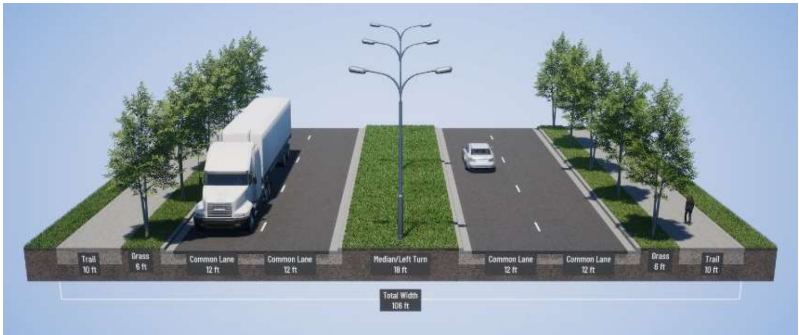
Figure 3.5 – Commercial Arterial Typical Section
