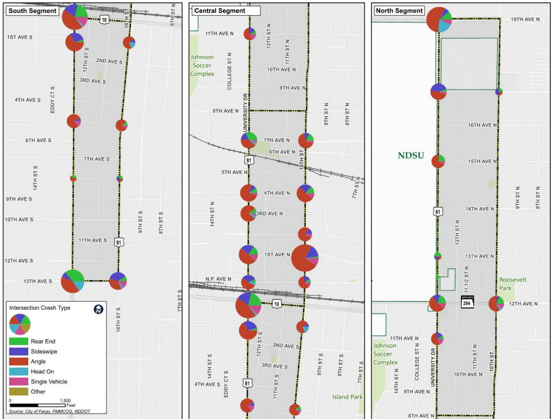
Figure 20: Intersection Crashes by Manner of Collision
