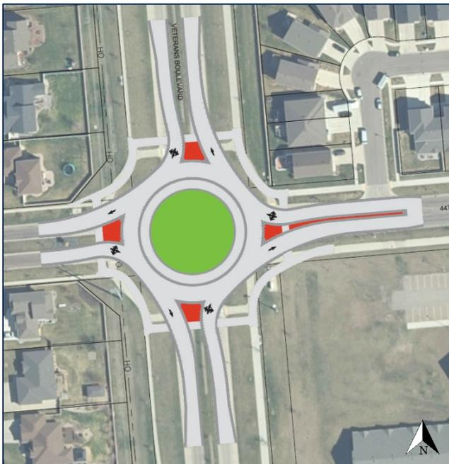
Figure 4: 150-Foot Roundabout Concept for Veterans Boulevard and 44<sup>th</sup> Avenue South
