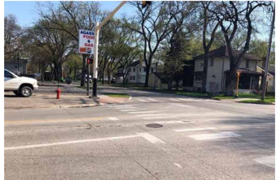
▲ Intersections with University Drive have wide curb radii and faded pavement markings.
