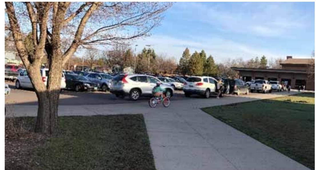
▲ There is no vertical separation between vehicle and pedestrian space, which results in drivers encroaching onto the sidewalk.
