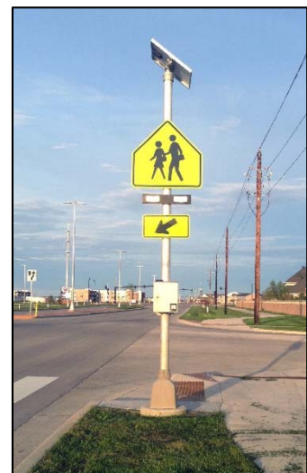
FIGURE VII-1: RECTANGULAR RAPID FLASHING BEACON ON 40 TH AVENUE NEAR SHEYENNE HIGH SCHOOL
