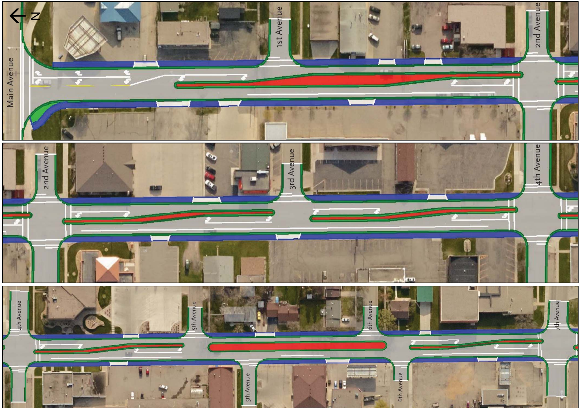
FIGURE V-17: CORRIDOR LAYOUT FOR TWO-LANE SECTION WITH TURN LANES AND RAISED MEDIANS ROADWAY ALTERNATIVE FOR SHEYENNE STREET FROM MAIN AVENUE TO 7TH AVENUE
