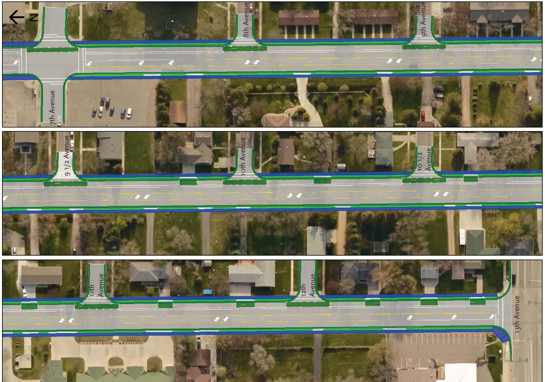
FIGURE V-28: CORRIDOR LAYOUT FOR SEPARATED BICYCLE LANES ROADWAY ALTERNATIVE FOR SHEYENNE STREET FROM 7TH AVENUE TO 13TH AVENUE
