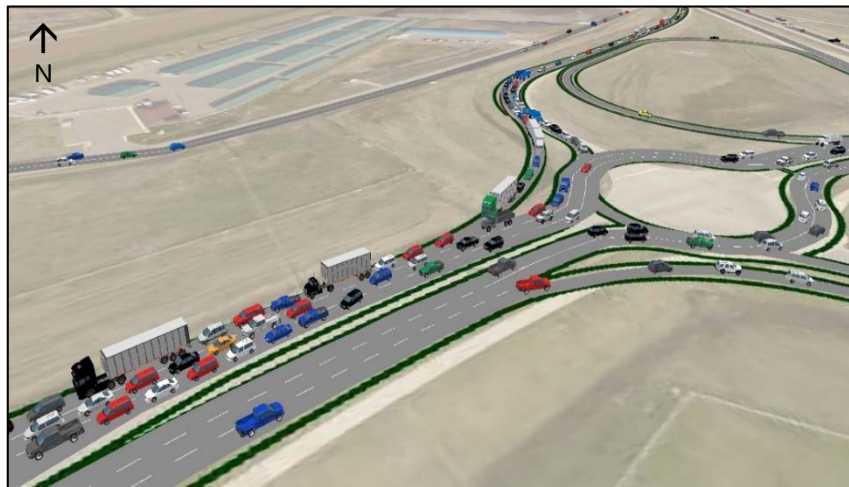
FIGURE VIII-15: ROUNDABOUTS WITH SOUTHWEST LOOP ALTERNATIVE FOR SHEYENNE STREET INTERCHANGE
