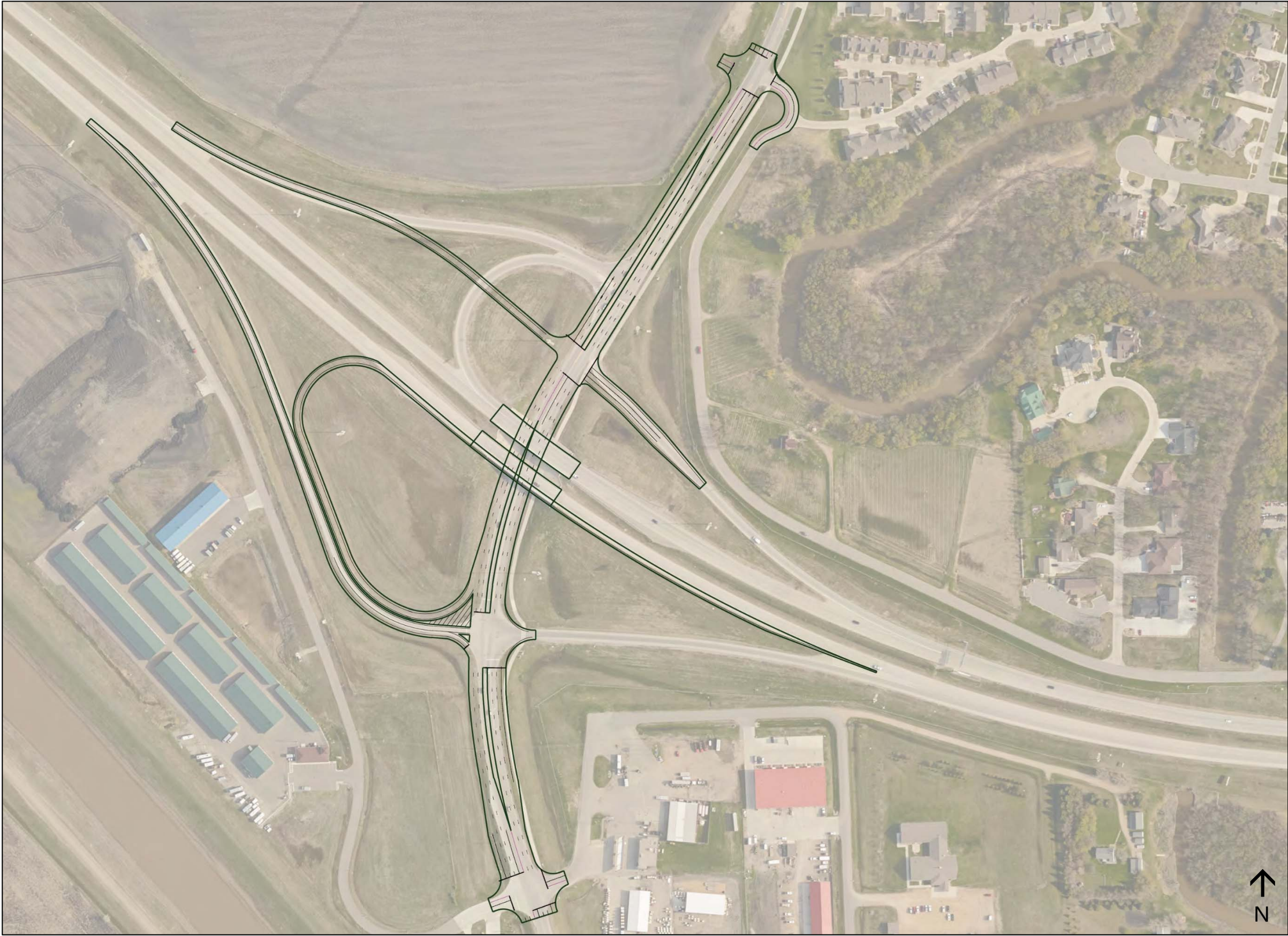
FIGURE VIII-4: NORTHEAST RAMP ALTERNATIVE FOR SHEYENNE STREET INTERCHANGE
