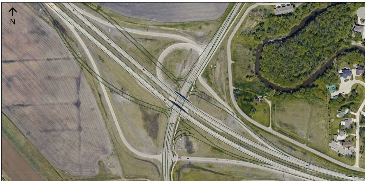
FIGURE VIII-13: SINGLE POINT URBAN INTERCHANGE ALTERNATIVE FOR SHEYENNE STREET INTERCHANGE
