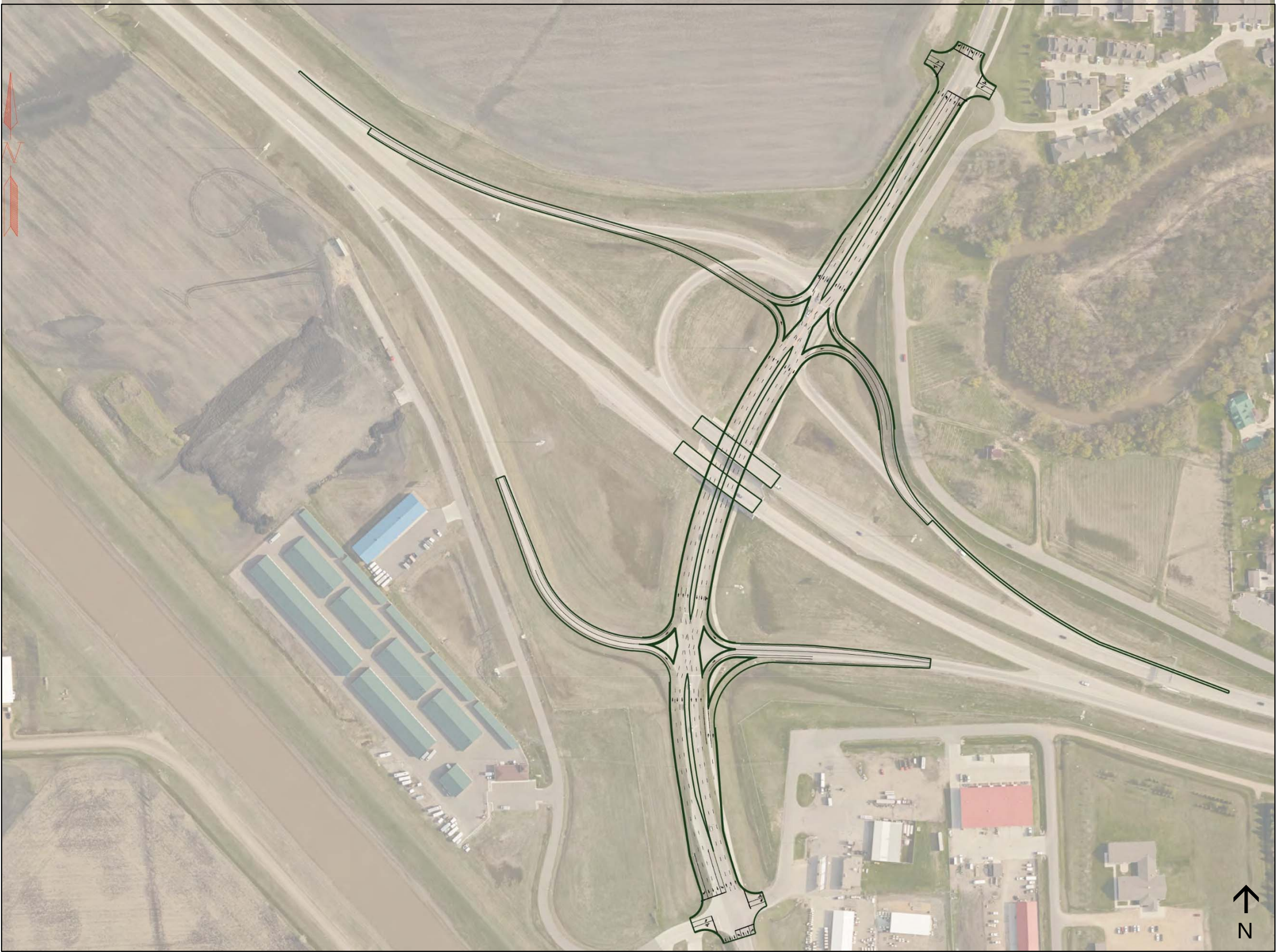
FIGURE VIII-10: DIVERGING DIAMOND INTERCHANGE ALTERNATIVE FOR SHEYENNE STREET INTERCHANGE
